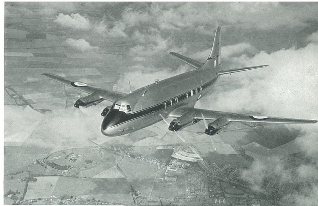
The first prototype Vickers Viscount flying with two engines feathered
