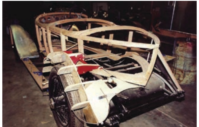
George Forbes 20hp chassis GOK74 showing the body under construction. Note the bucks for the mudguards.
